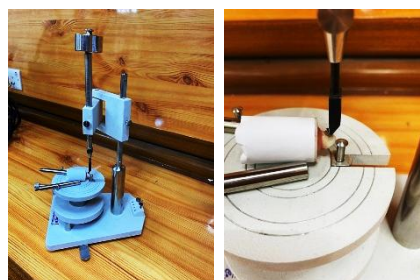
Figure (4): Gerdent Surveyor with a load of 200 gm. to standardize the pressure for all the specimens.
