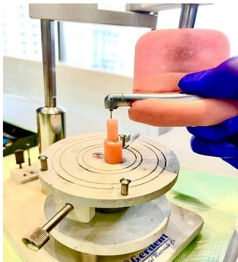
Figure (4): Application of a laser on an acrylic surface
