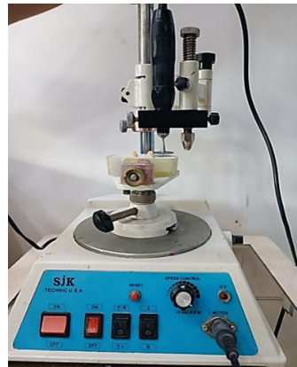
Figure (2): A milling machine used for cutting the ridge lap portion of synthetic teeth
