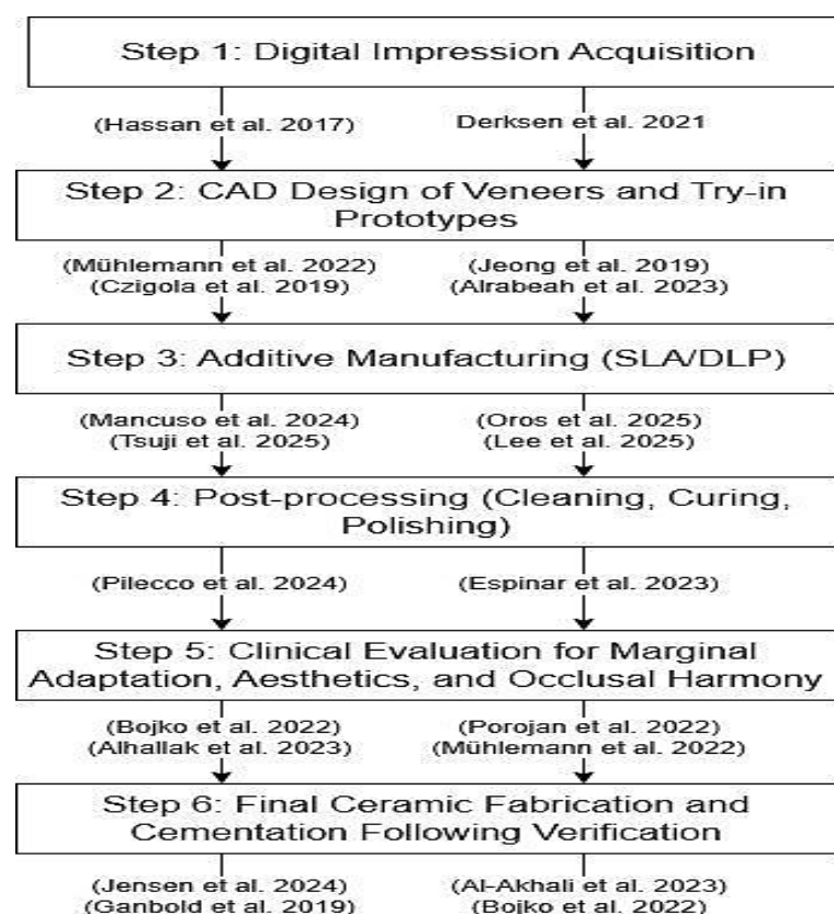
Figure (2): Workflow diagram of 3D printed try-in fabrication and clinical validation
