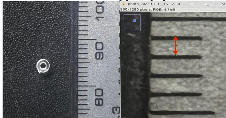
Figure (3): (A): Photographs using a millimetric ruler of vernier caliper (Richmeters, Ningbo, China), (B): pixel value of 1mm in the ImageJ software
